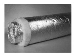
The **SONODEC**® series consists of a perforated aluminum laminate inner duct, a polyester barrier to prevent the diffusion of glass wool particles, thermically and acoustically insulated with a glass wool layer and provided with an outer jacket strengthened with glass fibre.
